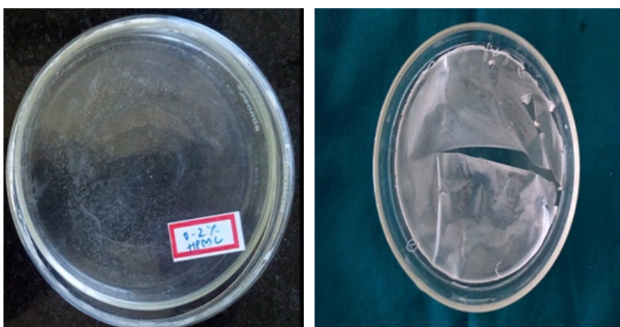
Figure 5: Fibroin solution with 0.2%HPMC and the final silk fibroin membrane
