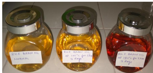
Figure 1 Normal and thermally oxidized rice bran oil at 100 and 180°C for 3 days
