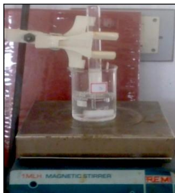
Figure 7: Open ended cylinder with dialysis membrane in simulated tear fluid pH 7.4
