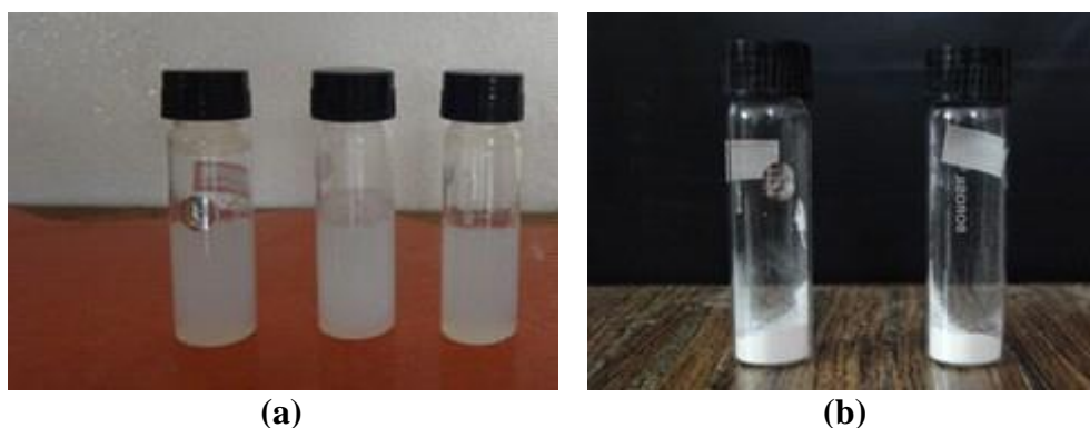
Figure 1: a) Norfloxacin nanoparticulate suspension; b) Freeze dried norfloxacin nanoparticle
