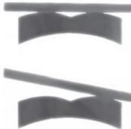
Figure 4: Rounded arch slot floor reduces friction since the archwire contacts the floor at only two points. Synergy®, RMO®
