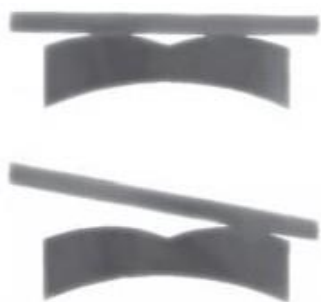
Figure 2: Rounded arch slot floor reduces friction since the archwire contacts the floor at only two points. Synergy®, RMO®
