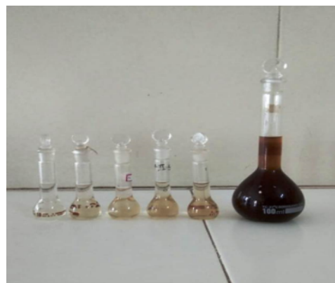
Figure 2: Formation of Ag-Nps of Aqueous Extract of Zingiber Over a 1-hour Time Period
