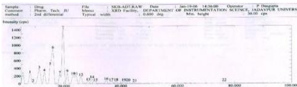
Figure 3a2: X-ray powder diffraction peaks of parent drug (Nateglinide)
