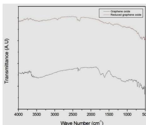
**Figure 4: FTIR spectra of graphene oxide and reduced graphene oxide**
