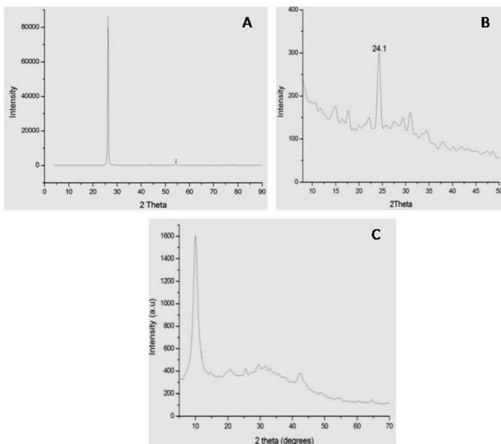
**Figure 3: XRD pattern of A) raw graphite B) graphene oxide C) reduced graphene oxide**
