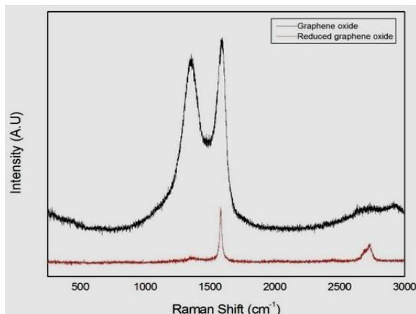
Figure 5: Raman spectra of graphene oxide and reduced graphene oxide
