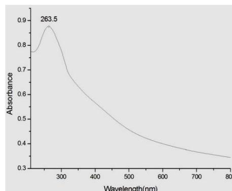
Figure 2: UV-Vis spectrum of oxide reduced graphene oxide
