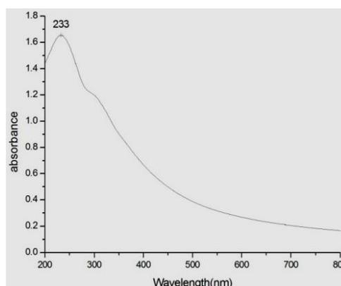
Figure 1: UV-Vis spectrum of graphene
