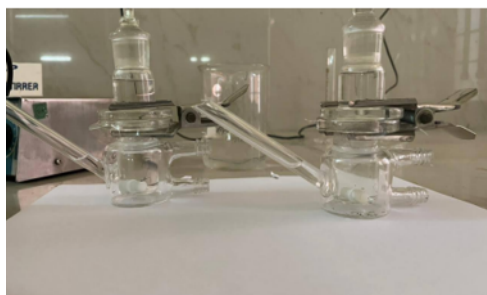
Figure 4: Franz Diffusion Cell Apparatus
