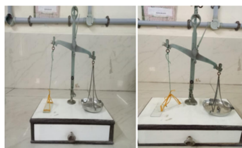
Figure 3: Spreadability Studies Done Using Weighing Balance
