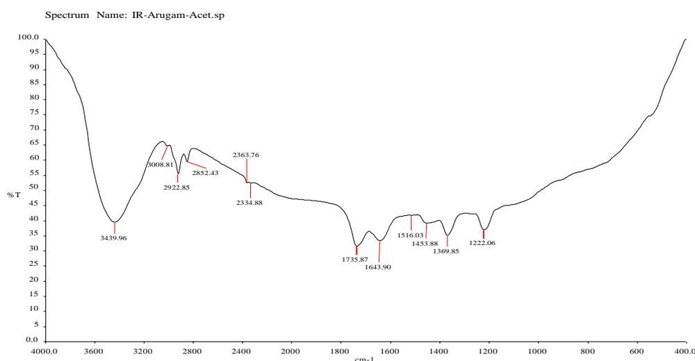
**Figure 2: FTIR spectrum of biosynthesized AgNPs using Cynodon dactylon**
