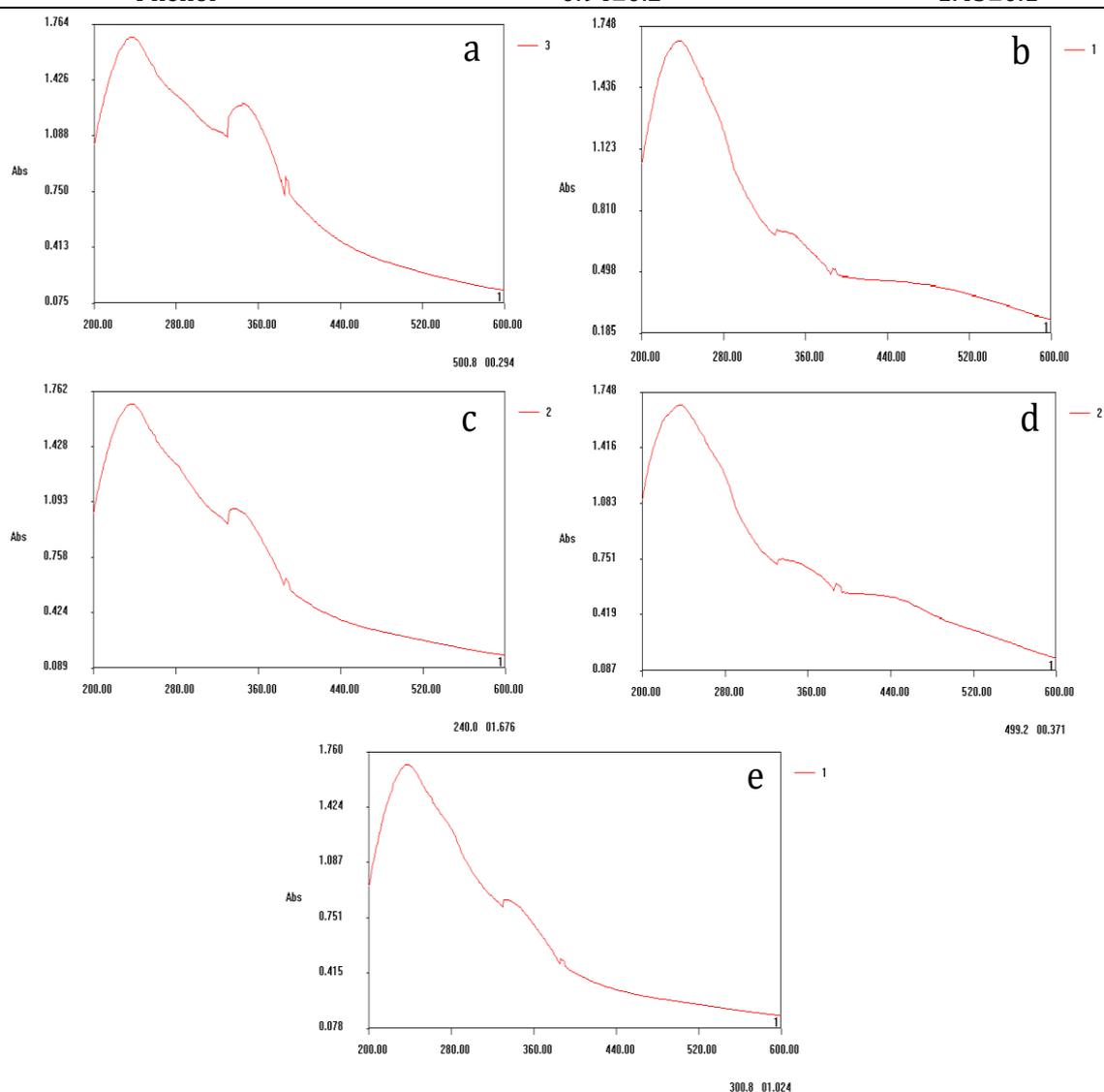
**Figure 1: UV-vis spectrum of synthesized silver nanoparticle a) 75°C; b) 60 min; c) pH-4; d) pH-8; e) 1mM**
