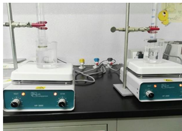
Figure 4: Modified USP XXI diffusion assembly
