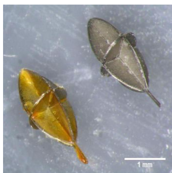
Figure 6: Microrobot utilizing functional coating; (Right) a bare magnetic microrobot made of thin assembled nickel pieces; (Left) a Microrobot coated with oxygen sensitive film
