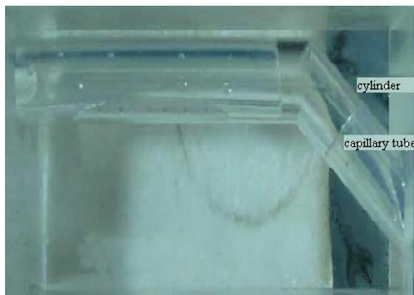
Figure 2: Fluidic manifold with an inner capillary
