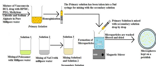
**Figure 2: Preparation of VLM by Double Emulsion method**
