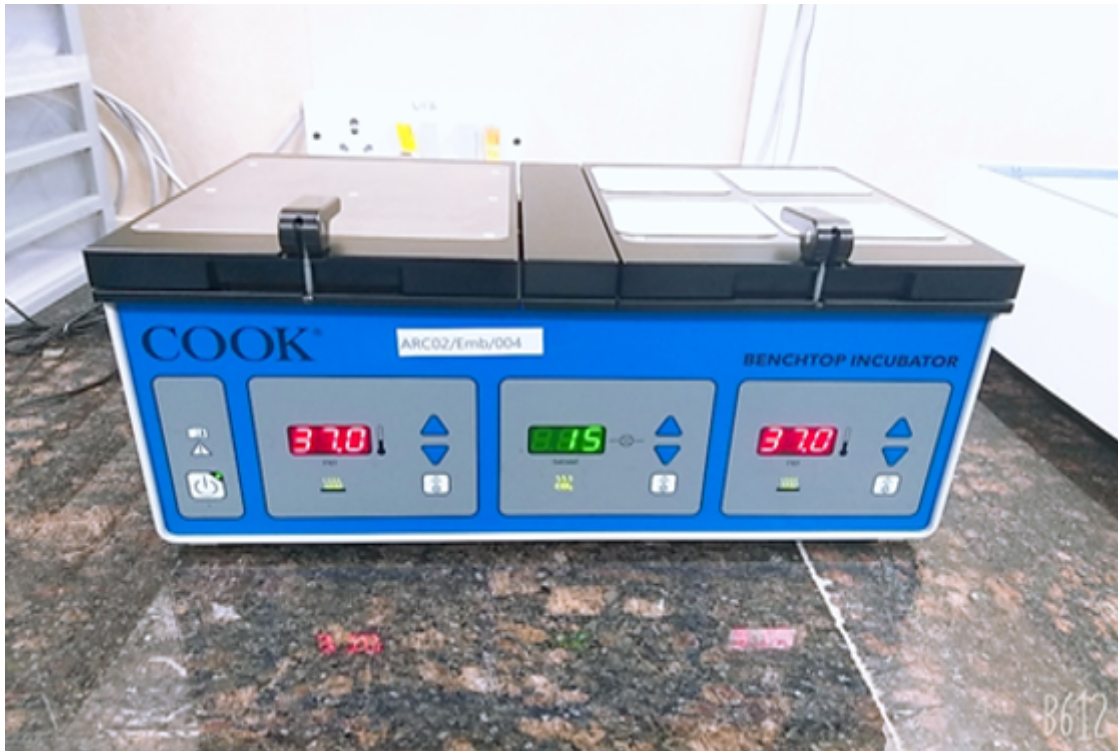
Figure 1: Benchtop incubator, COOK-K- Minc (humidified)
