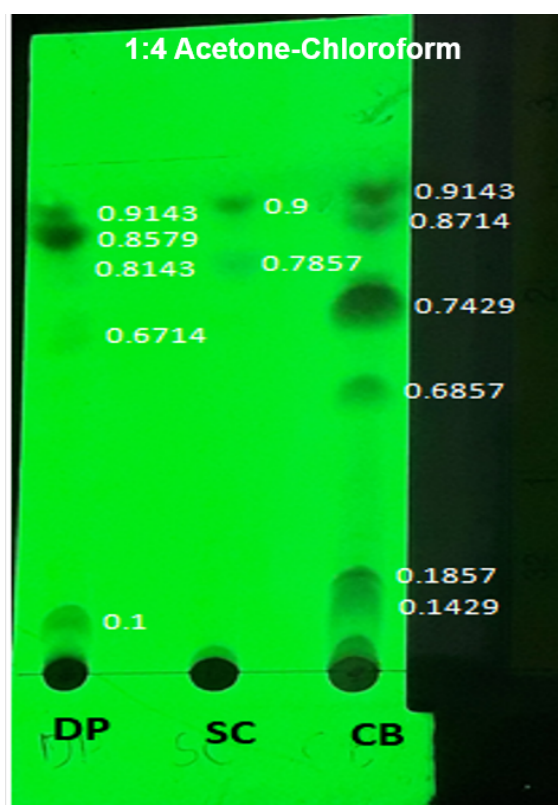
Figure 3: Thin Layer Chromatography Plate under 254 nm
