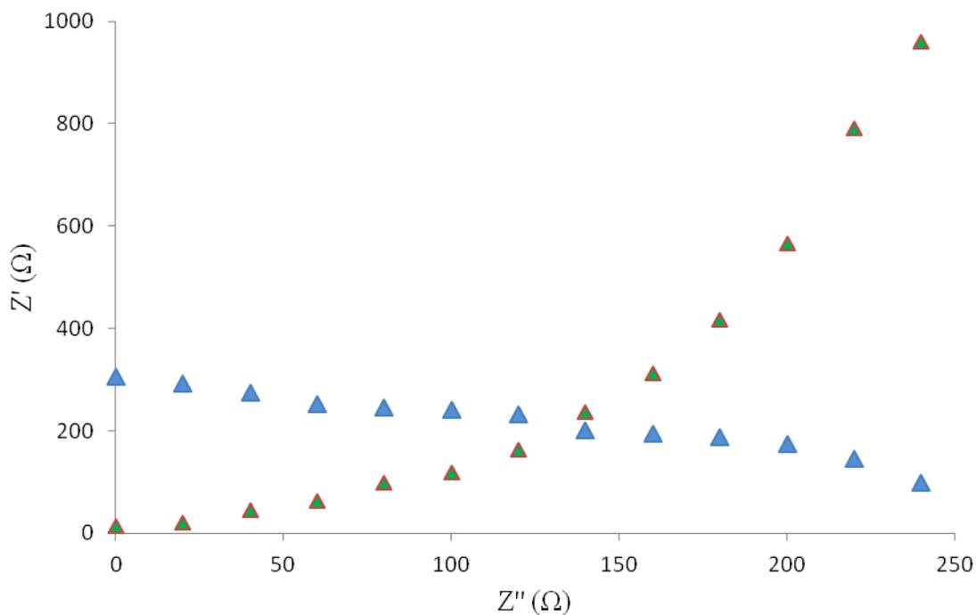
**Figure 3: Nyquist plot of Electrochemical Impedance Spectroscopic of free NaR and NaR Nanoparticles coated Au electrode.**
